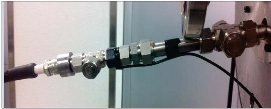
Figure 29 - Modified spark plug in ignition system set up
